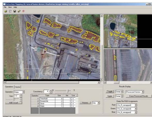
Fig. 9. IKONOS imagery has been fused and combined with spatial context features for mining. A first-time user rapidly trained the system to search for iron ore. This detection mapping capability is part of the Image Mining module and supports morphological filtering of the detections and conversion to vectors for map-making. Iron ore detections have been outlined by vectors in yellow, and train cars are found carrying ore to the plant (as revealed in the lower-right detail window). (IKONOS imagery provided by ERDAS/Leica Geosystems.)
