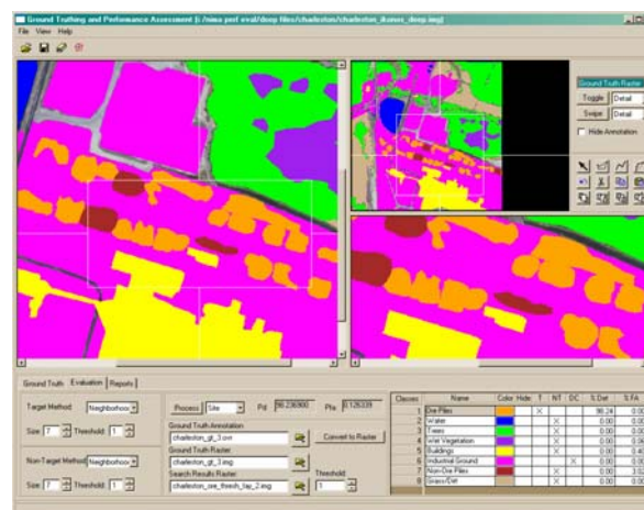
Fig. 10. The Ground Truth and Performance Assessment module is used here to evaluate detection performance for iron ore extraction in this Charleston, South Carolina IKONOS scene. The ground truth classes are shown in pseudo-color, and the results of the performance assessment are displayed in text fields on the tab window.
